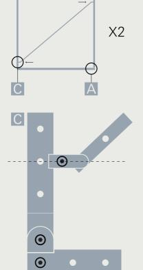
slide the four cross-rails onto the centre cross – all five screw heads should face the same direction. to secure cross, turn the small screws counterclockwise from inside of the rail (D). only turn until first resistance, then another 1/3 turn. overtightening might damage threads.
