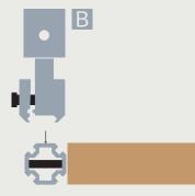
use the clamps to assemble one supporting beam between each leg pair, again with outward-facing screw heads. align the clamp with the second hole on the lower side (C). also note where the logo is placed on the right side (A).
