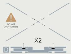
place the cross-assembly on the correct side of the desk (E) and fasten with the two lower clamps. take your time to align the clamps with the second hole of the rail (F). adjust the legs on both sides when tightening the two upper clamps, to a straight 90° angle.
