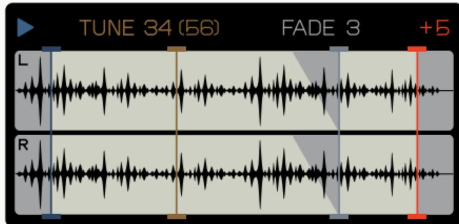
this is a zoomed in view, great for adjusting exact in and out zero positions within the sample. tap any encoder to zoom in around its section. tap again to exit to the main view.
