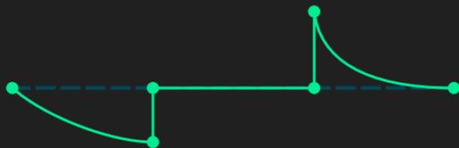
Dynamic Envelope is specially designed for short drum sounds. Set the attack level with Blue Encoder, Mid part level with Green Encoder, Release Level with Encoder and use the Orange Encoder to adjust the region.
