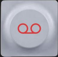
Your OP-1 has a built in tape feature with 6 minutes of recording time (in normal tape speed and 44.1 kHz/16 bits). It has 4 individual tracks. To enter the Tape Mode press the Tape key with the orange tape symbol on it.
