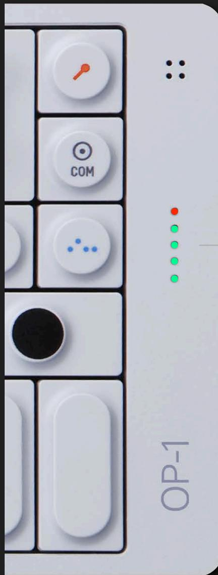
The Battery level is indicated by the LED array on the right side of your OP-1. All LEDs lit (including the red) indicates a fully charged battery good for around 16 hours of heavy use. The stand-by time is approximately 2 years.
