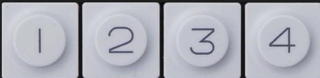
NOTE: The T1-T4 are soft keys, which means that in Synthesizer and Drum mode they function as described here. In Tape mode they are track keys T1-T4 and in Mixer Mode they are Mixer (T1), EQ (T2), Master Effect (T3) and Master Out/Drive (T4).
