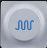
To enter Synthesizer Mode, press the key with the blue wave symbol on it. This enables both T1-T4 and sound selection keys 1-8.
