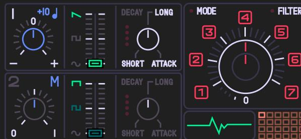
DBOX, short for DRUMBOX, is a dual oscillator synthesizer, convenient for producing drum sounds. Blue encoder adjusts pitch, Green encoder adjusts waveform, White encoder adjusts envelope. Hold SHIFT to access secondary oscillator. Orange encoder is used for Cross Modulation and, when SHIFT is pressed, Filter cutoff frequency.
