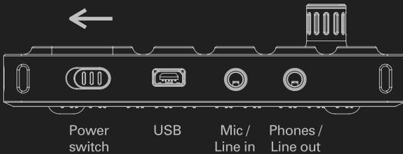
To power off, slide the power switch away from you. Data is always stored on-the-fly, so you don't have to worry about saving your sound or recordings.
