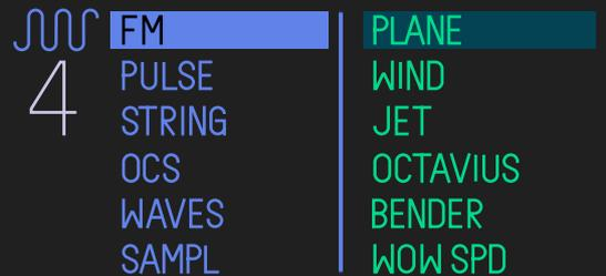
NOTE: The difference between changing just a Synthesizer Engine (SHIFT + T1) and a Sound (SHIFT + 1-8) is that the later changes all four T1- T4 settings.
